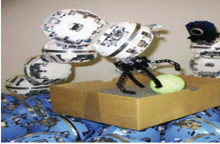
FIGURE 1: Lattice type architecture [20] (copyright @ 2007 Brandt et al.).
